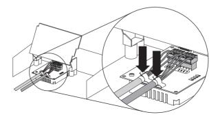
18. Screw the nuts tightly onto the cable gland to fix the cable.
