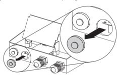
Unscrew counter nut from the delivered cable gland.
