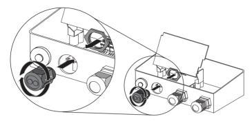
$\square$  The cable opening on the inverter is prepared.
