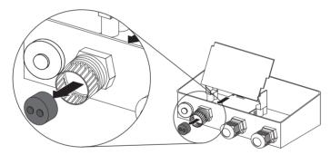
Remove 1 or 2 filler plugs from the cable gland.
