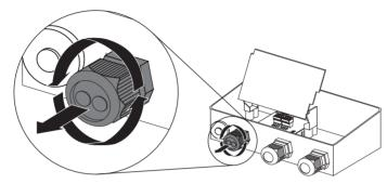
9. Press the seal out of the cable gland from the inside.
