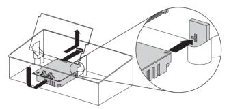
7. Secure the module with the screw.
