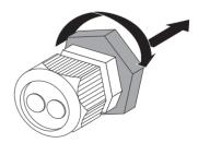
Place the cable gland into the enclosure opening of the inverter and fastening it along with the counter nut from inside.
