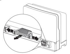
3. Loosen the screw of the display, until the display can be flipped up. Flip up the display until it clicks into place.
