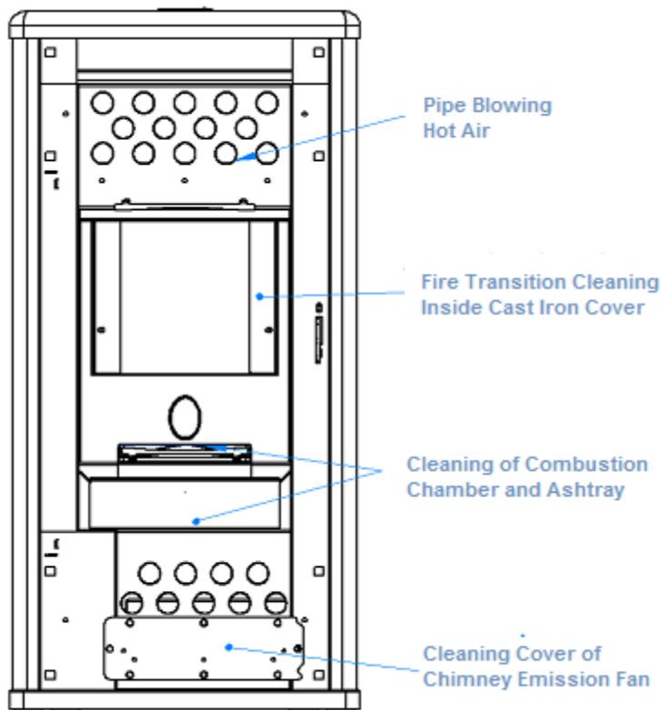
Once a year, stove fire transition pipes are cleaned through moving out cast iron cover and cleaning cover of chimney emission fan
