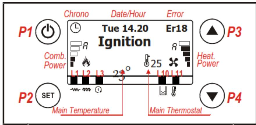
The main display shows; date, hours, chrono activation, combustion power, heating power, functioning state, possible error code, main temperature and main thermostat.
