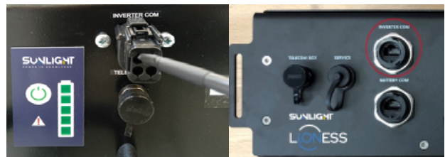
Picture A1.3 Inverter's Communication cable with Li.ONESS Power / PBT Unit (Battery Side)
