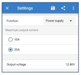
It is also possible to enable low current mode while in power supply mode and to specify the desired output voltage.
